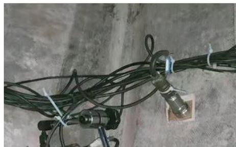
图3 道床测点布置
